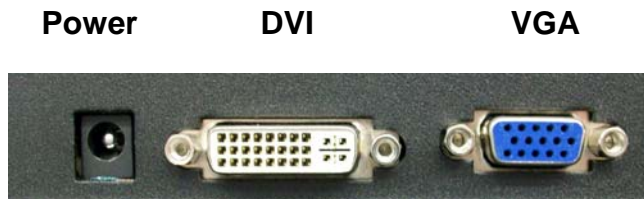
Above Illustration – Interface Connections (Rear Entry)
